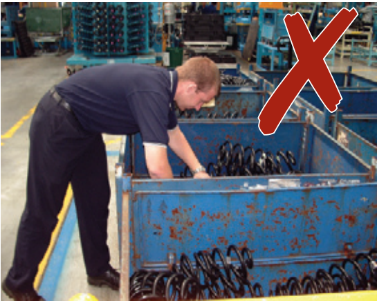
Bending into stillages on the ground is hazardous for your back.
