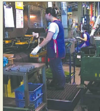
This platform raises the worker up to a better height.
